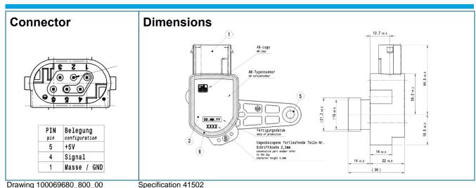
IP 6K9K (with fitted Output - voltage (0.5 ... 4.5) V Supply Sealing grade female connector) range Temperature -40 °C to 100 °C ± 45° **Output signal** Angle range 1 signal (analog) range AMP No. 114-18063-21 (coding A) Current gold plated, Independent linearity ≤ 1 % Max 5.5 mA Connector consumption Female connector on request
